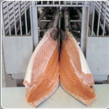
Splitting with removal of backbone only
